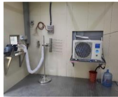
OUTDOOR AC CHAMBER ADJUSTMENT AND WB / DB (WET BULB AND / DRY BULB APPARATUS)
