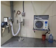
OUTDOOR AC CHAMBER ADJUSTMENT AND WB / DB (WET BULB AND / DRY BULB APPARATUS)
